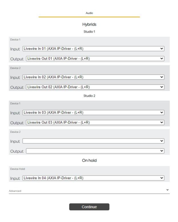
In this example, Studio 1 has had two audio devices configured and Studio 2 has been deliberately assigned only one on-air audio device.
