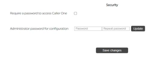
REQUIRE A PASSWORD TO ACCESS CALLER ONE UNCHECKED = USERS DO NOT NEED A PASSWORD FOR THE MAIN SYSTEM, BUT ADMINS DO FOR THE CONFIGURATION AREA.
